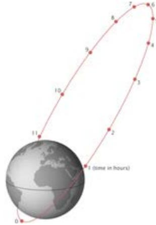
**Figure 14. An example Molniya orbit, with the satellite's location in the orbit marked in hours from perigee. Image from Wikimedia Commons ([source](#))**
