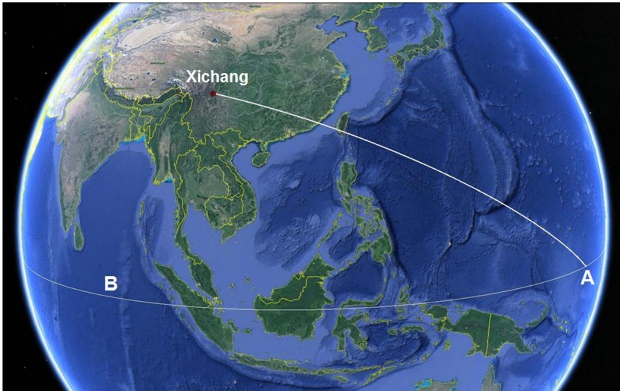
**Figure 11. The ground track of a rocket from Xichang for a non-rotating Earth indicated by Point A and a rotating Earth indicated by Point B ([source](#)). Image © 2013 Google Earth.**
