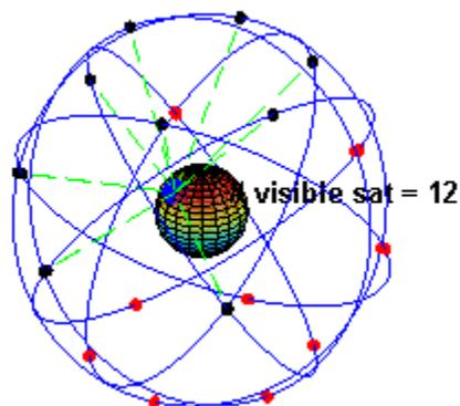
**Figure 13. A notional 24-satellite GPS constellation and the number of satellites visible from a ground location at 45 degrees north latitude. Image from Wikimedia Commons ([source](#))**
